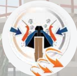
STAGE 2 - CONE CRUSHER
